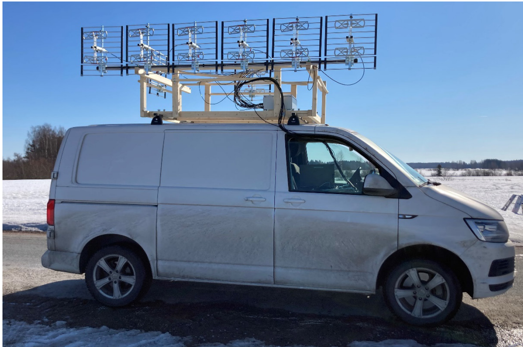
Figure 1: Car-mounted passive radar system.
